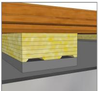
KTL SPORT MULTIFLEX ADVANCED is an area-elastic sports floor, based on 22mm solid hardwood 2-strip parquet boards, nailed to a resilient 1-layer batten system, installed floating on levelled concrete or wooden based subfloor. Total construction height incl. floor board is 52mm.
