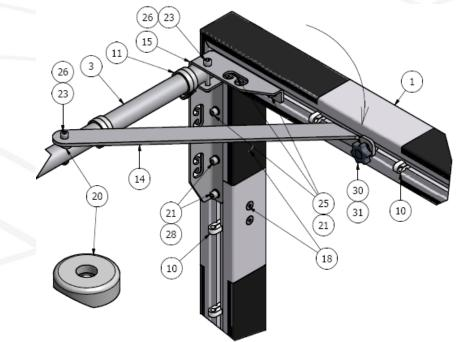
5. Place the net to the goal installing by installing the net hasps (10) and hitches (11) according to the diagram and interspersing the top rope in the rings placed in the top corners of the C-shaped pipes (3).
