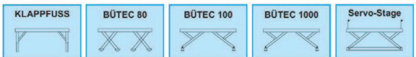
Platforms that can be adjusted to multiple heights in intervals of 20 cm; custom heights are available.
