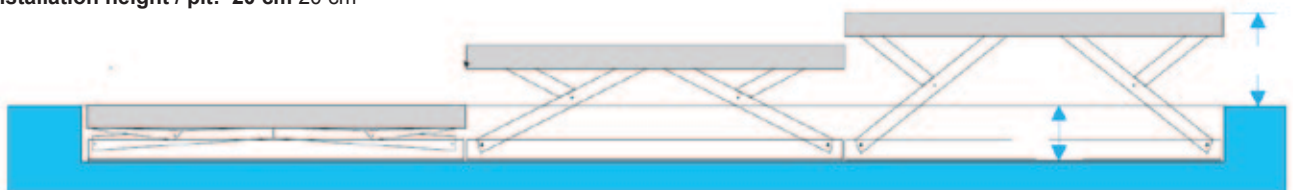
The Servostage can do everything: It remains on the ground level, raises step by step or forms an elevated platform.
