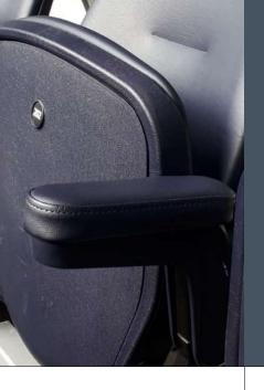
deluxe is a more substantial armrest, its fold back function allows it to be used on telescopic platforms, folding automatically on contact with the deck.
